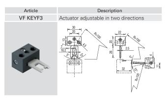
Actuator adjustable in two directions for guards with reduced dimensions.
