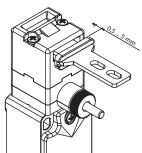
The actuation head of this switch features a wide range of travel. In this way the guard can oscillate along the direction of insertion (4.5 mm) without causing unwanted machine shutdowns. This wide range of travel is available in all actuators in order to ensure maximum device reliability.
