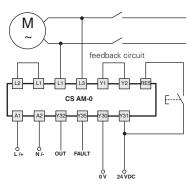
$\bigwedge | \bigwedge$  In case of star/delta starting, connect the module to the ends of a single winding For dc motors connect + with L1 and - with L3.
