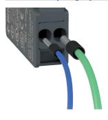
The PUSH-IN spring connection allows quick and simple wiring, as the wire just needs to be inserted into the appropriate hole in order to establish the electrical connection and automatically secure the wire. The reduced force required to insert the wire allows completely toolfree connection by using wires with crimped wire-end sleeves. They are released by pressing a special wire release button - including individually - with any tool, without the need to use a screwdriver of a predefined size.
